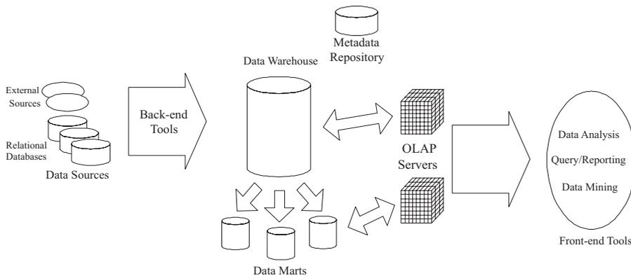
**Fig. 1.1.** Data Warehouse architecture
